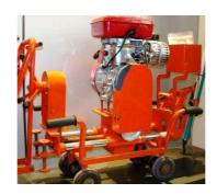
**INTRODUCTION**: - Light Weight Rail Drilling Machine is an efficient machine in hands of permanent way inspector which facilitates him with an easy drilling method while making holes in different types of rails. The machine requires the need of only two semi-skilled gang men. The Mono Rail Wheel assembly helps the machine to get carried away on track as well as on cess from one place to another at different sites in no time.
